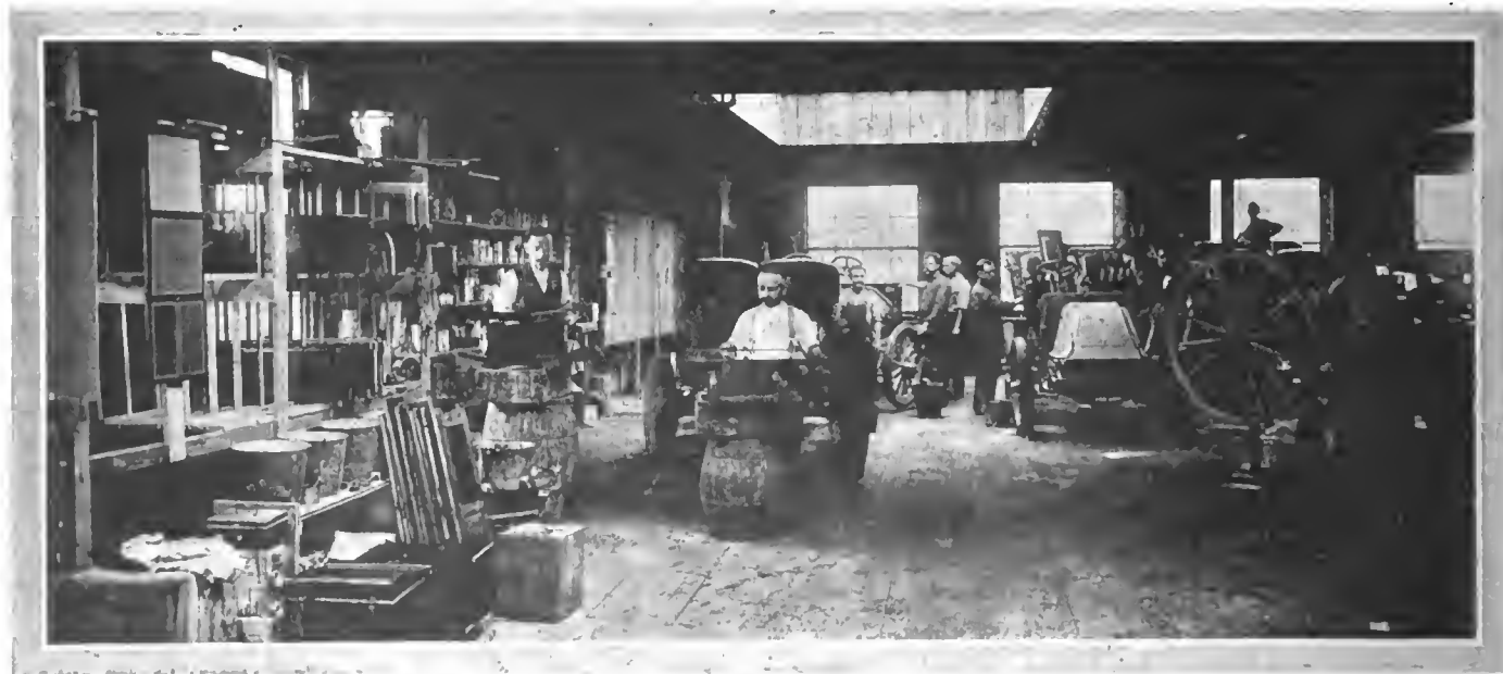
A GENERAL VIEW IN THE PAINT SHOP, WHERE EACH AUTOMOBILE RECEIVES TWENTY COATS.
